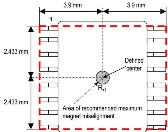
Figure 18: Defined IC center and magnet displacement radius
