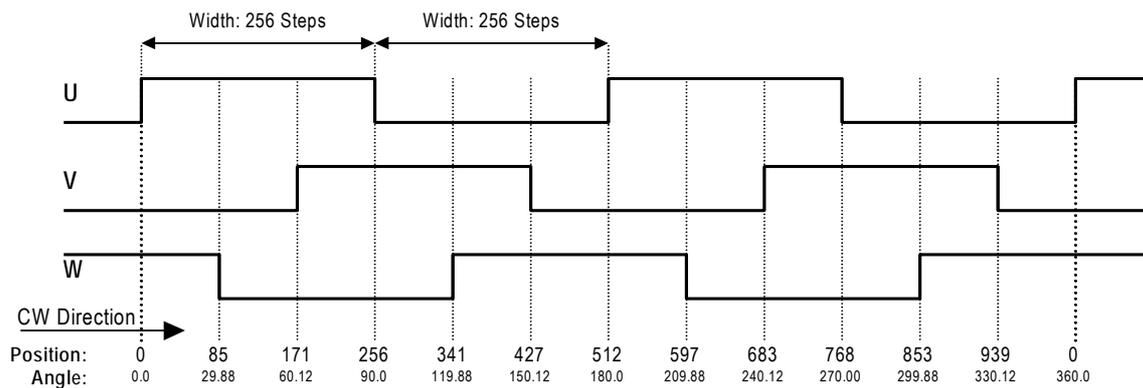
Figure 12: U, V and W-signals for 2pole BLDC motor commutation (Div1=1; Div0=0)
