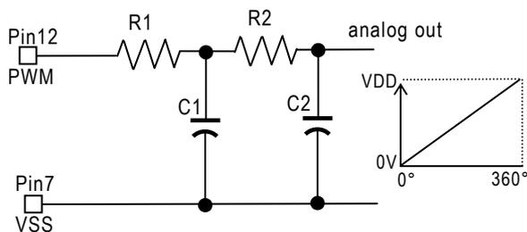
Figure 10: Simple passive 2<sup>nd</sup> order lowpass filter
