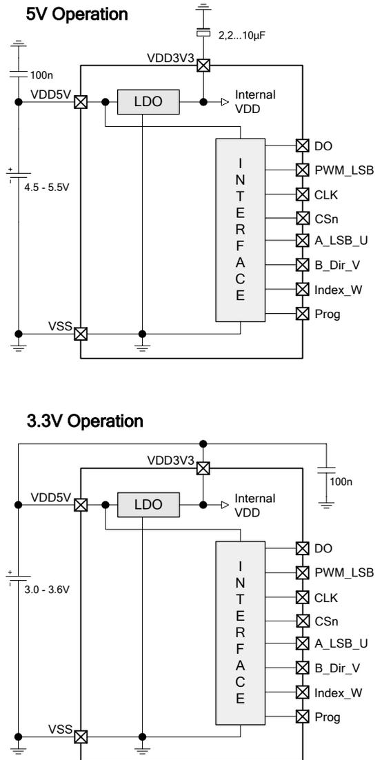
Figure 16: Connections for 5V / 3.3V supply voltages
