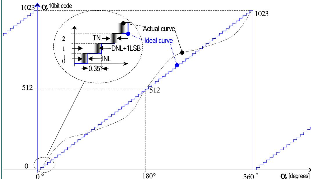
Figure 23: Integral and differential non-linearity example (exaggerated curve)
