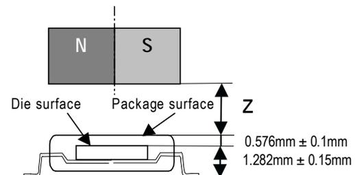
Figure 19: Vertical placement of the magnet
