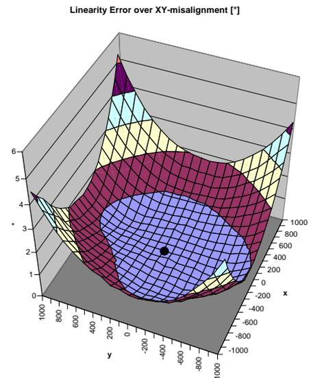
Figure 21: Example of linearity error over XY misalignment
