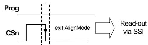
Figure 15: Exiting alignment mode
