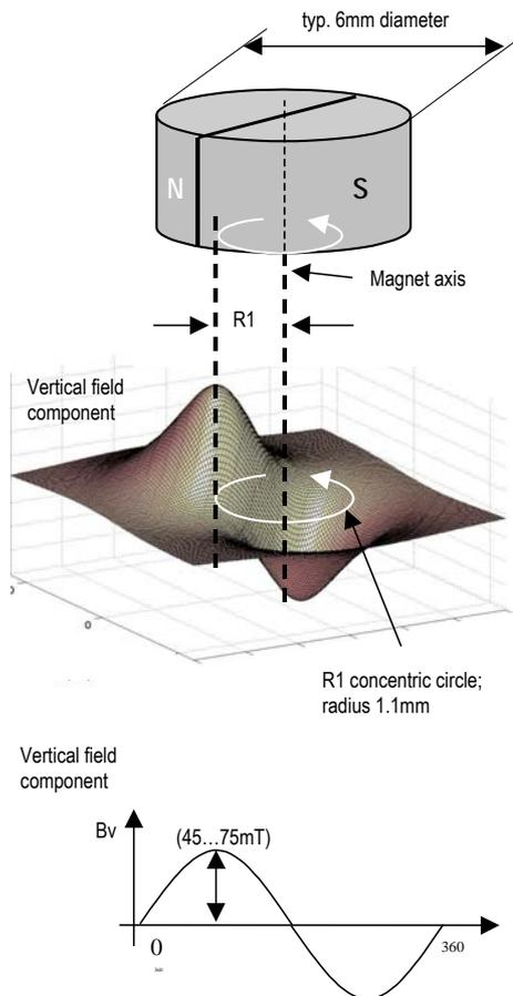
Figure 17: Typical magnet and magnetic field distribution
